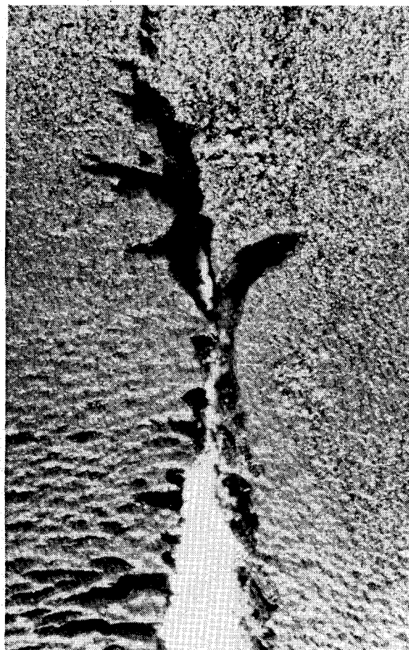
Fig. 7a Front view of recovered sample exhibiting mode C crack propagation and branching (same magnification as Fig. 2b).
